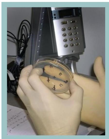
Researchers at Purdue's Biometric Standards, Performance and Assurance Laboratory test bacteria from a vein-recognition reader, a biometric device that can authenticate a person's identity. Researchers have found that although the surfaces of some biometric devices may look more unsanitary due to visible dirt and prints, they harbor about the same amount of bacteria as a typical doorknob.
